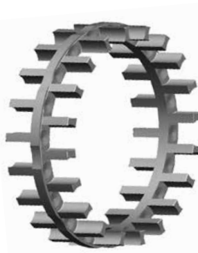
Fig. 5. One-piece finger-type cage.
