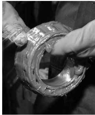
Fig. 15. Grease can easily be packed by hand.
