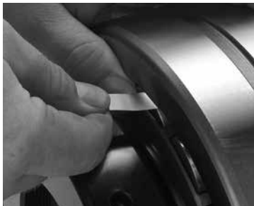
Fig. E-7. Measure RIC before installation.
