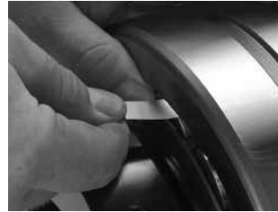
Fig. E-3. Measure RIC before installation.
